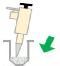
9. Transfer the mixture back to the Seed Bead tube. Repeat the process until no crystals are visible in the drop.
