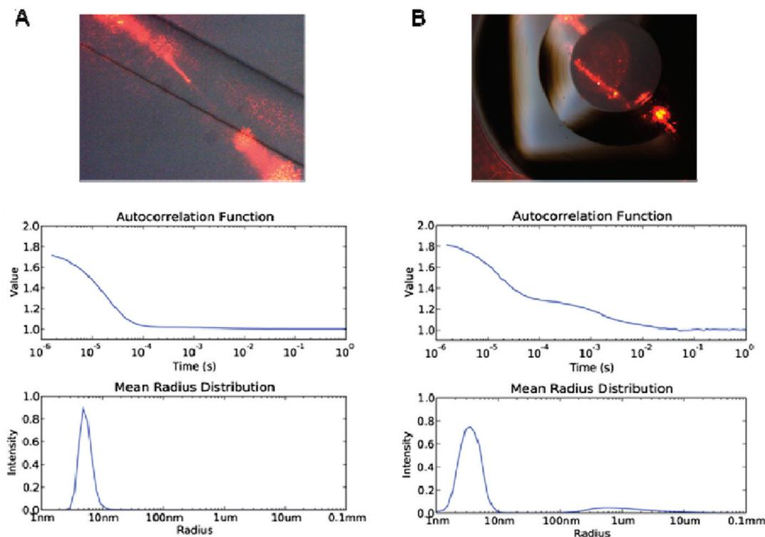
**Figure 4.** (a) DLS *in situ* measurement in a capillary counterdiffusion crystallization experiment with glucose isomerase. Below is the corresponding autocorrelation function and radius distribution, and on the right (b) an *in situ* DLS measurement of a microbatch lysozyme crystallization experiment is shown.
