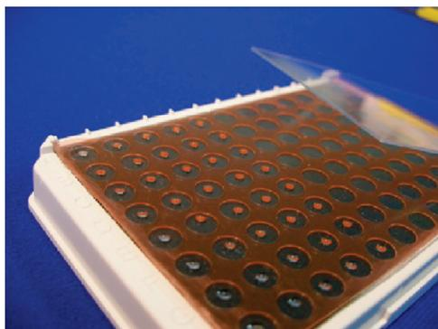
**Figure 8.** Laminex is a plate for crystal growth experiments, which occur in the narrow space between two plastic sheets or films. Laminex can be exploited with free interface diffusion, vapor diffusion, and microbatch.
