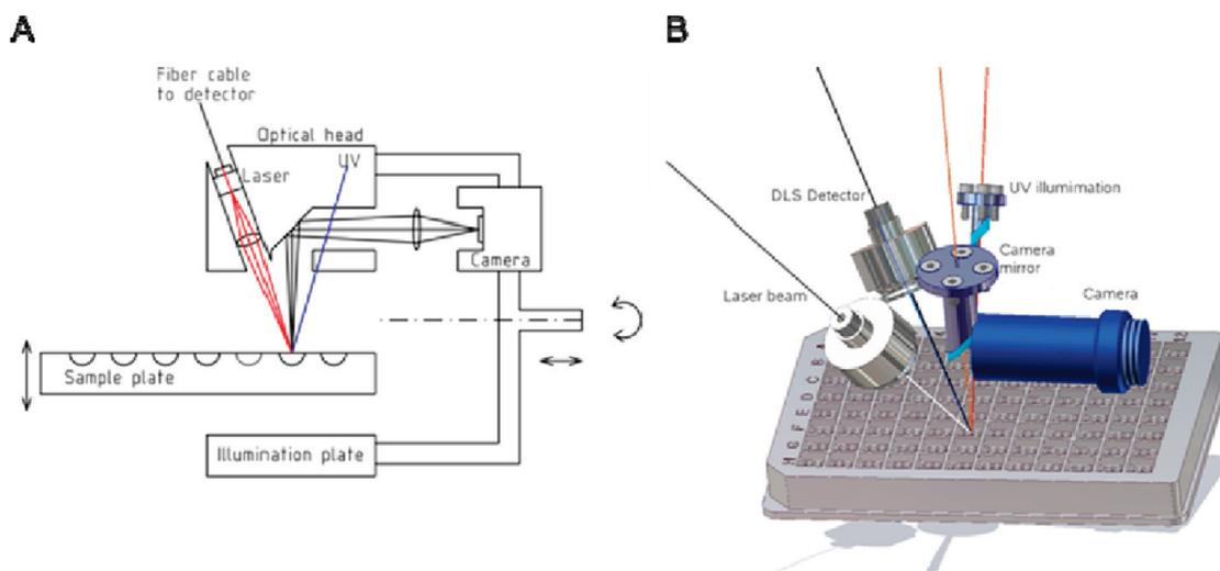
**Figure 3.** Scheme showing the *in situ* DLS imaging system named SpectroLight 500 and a close-up of the optics to analyze crystallization droplets in multiwell plates and other crystallization compartments. The hardware is manufactured by Nabitec GmbH and marketed as the Spectrolight 500 series by Molecular Dimensions Ltd.
