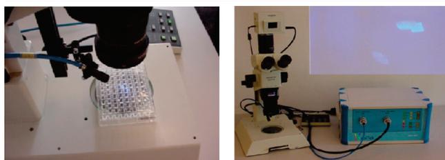
**Figure 6.** X-taLight 100, which offers a UV-fluorescence source and is shown attached to a microscope.
